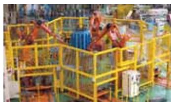
*Robotic Stator Core Lamination Stacking*
